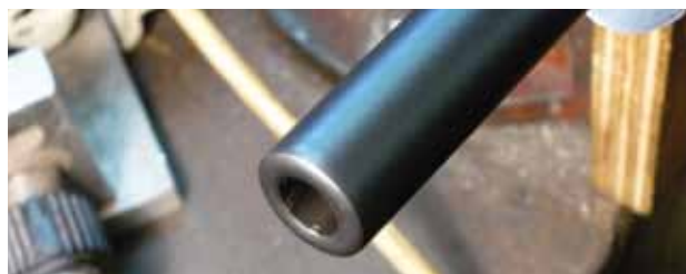
Shows rough factory crowning job with large gouges on the rifling lands from lathe tooling.
