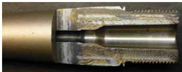
Shows 'section' of a factory barrel at chamber end. For best accuracy the machined throat section must be perfectly concentric in order to give the bullet a good straight start into the rifling.
