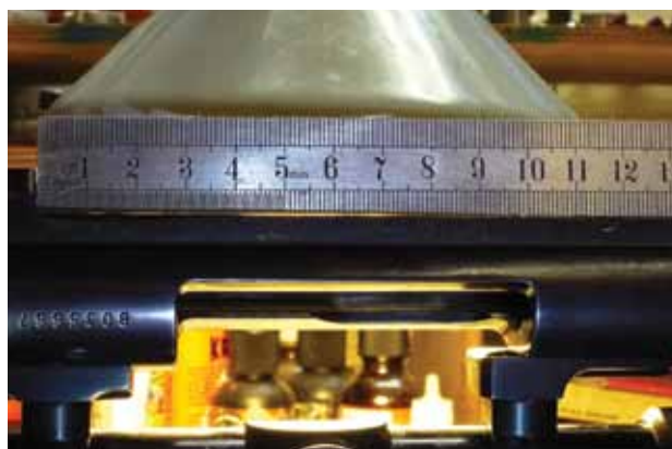
Straight edge along bottom of factory actions shows up warping due to heat treating when viewed against light source.
