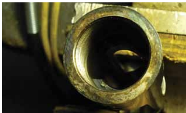
Factory receiver face roughly ground and not machined. Bluing is showing on no-contact areas. Often the receiver face is not 'square' with the receiver threads.
