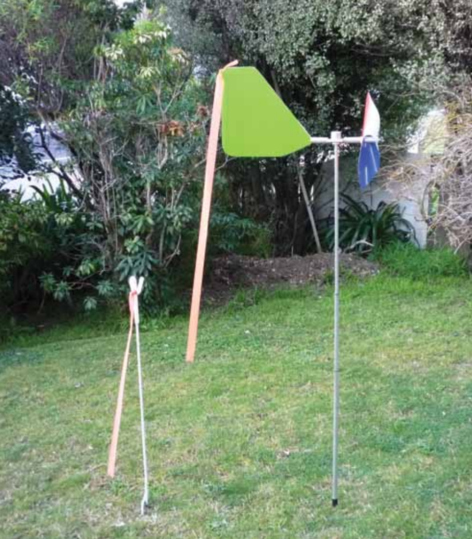
Wind flags are essential for accurate shooting, so that you can time your shots to occur in the same 'wind condition'. Professional flag on right is made by Ian Owen of Dunedin. Basic wind flags (shown on left) can be made from electric fence standards and surveyors tape/ribbon.
