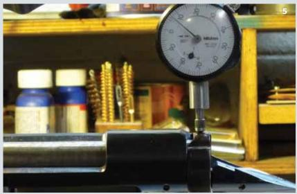
Sloppy bolt/action fit total 0.007" of play. Probably no issue on a bush rifle, but can cause frustrating flyers or vibration issues on a target or varmint rifle. This problem can be solved with gunsmithing. Sometimes in these cases, the bolt contacts only on one lug.
