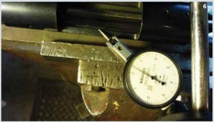
A very heavy barrel fitted to a lightweight sporter action – here you can see the twisting stress exerted on the action when the barrel is free floated. The deflection on the weak side-rail measures 0.0003" on this action which has a 25" barrel, weighs approximately 6lbs and has an outside muzzle diameter of 0.885". If a 32" long 7lb barrel was fitted this deflection would be even worse.
