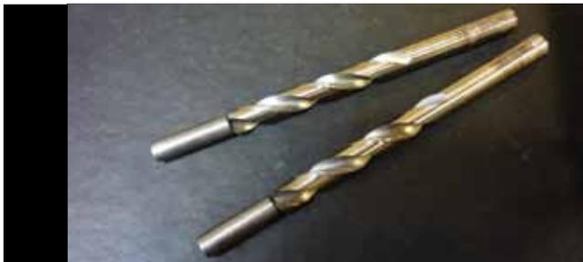
Pillars are drilled out with purpose-made piloted drill – this is to ensure adequate action screw shaft clearance. Shown are drills for 6mm or 1/4" pillar holes for action screw shaft clearance (action screws much not act as a 'recoil lug').
