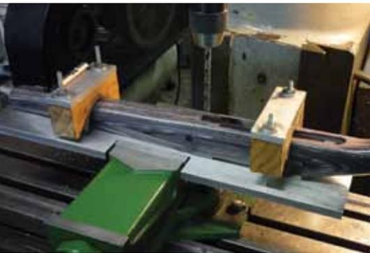
*Stock is drilled on special jig for pillar clearance*
