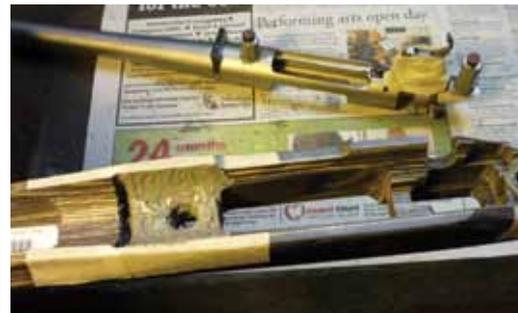
*Stock and metalwork prepped for bedding, tape on recoil lug front face and sides, release agent applied. We don't want a permanent 'glue-in'!*
