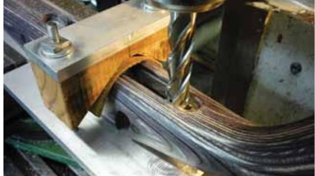
Metalwork cleaned down, excess compound trimmed off and stock tidied up. Bottom of pillars milled down to correct final height.
