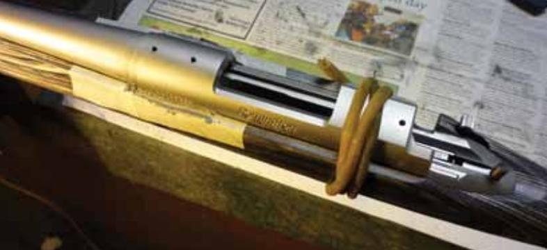
Allow to set. Magazine box must have clearance and should never be pinched tight. Barrel completed free floated on this model (sported barrel), and set at 'half depth' in the stock.
