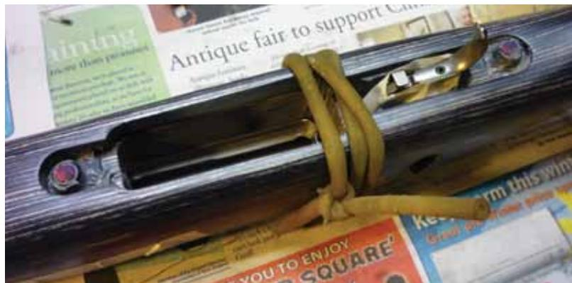
*Metalwork bought down into place, secured very lightly with surgical tubing, checked for correct alignment and then allowed to set overnight. Bedding of pillars must be done at the same time as the rest of the action for a perfect fit. Attempting to do a bedding job in two or three stages is a recipe for complications.*
