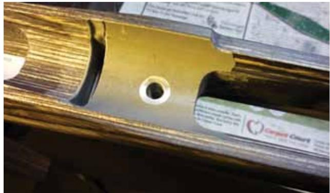
Action screws removed and metalwork carefully withdrawn from stock. Note no air pockets and a clean professional looking finish. The right release agent will assist greatly in achieving this. Top edge of compound can be stained to match walnut stocks if desired, and any exposed wood sealed. On fibreglass stocks the non-action-contact areas may need to be painted.
