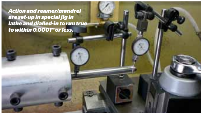
Action is ready to be 'trued' in special jig now with reamer/mandrel removed.
