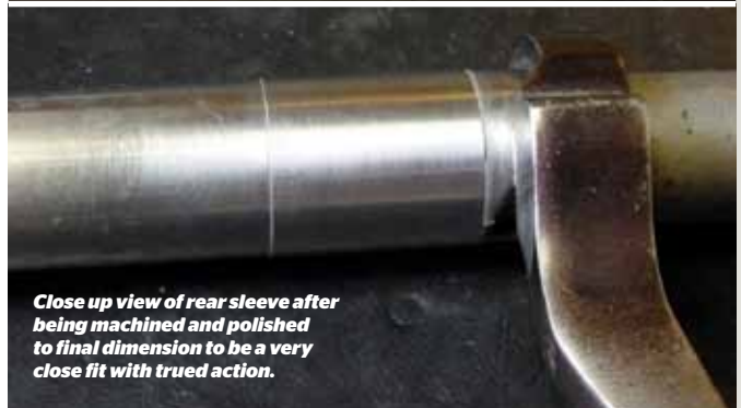
Sleeves are shown after being bonded to the bolt body.
