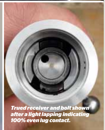
Perfectly centred firing pin strikes every time - evidence of a perfectly trued action, sleeved bolt, and precision-fitted rifle barrel blank.
