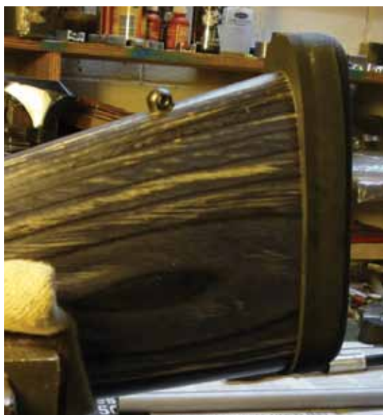
Install the (oversized) pad to the butt-end of the stock, and recheck that the pitch angle will be correct when finished.
