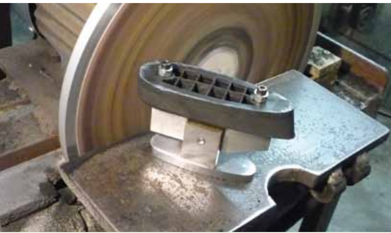
Set-up on special grinding jig.
