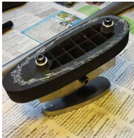
Mark outline with a scribe, taking care not to mark the stock finish.
