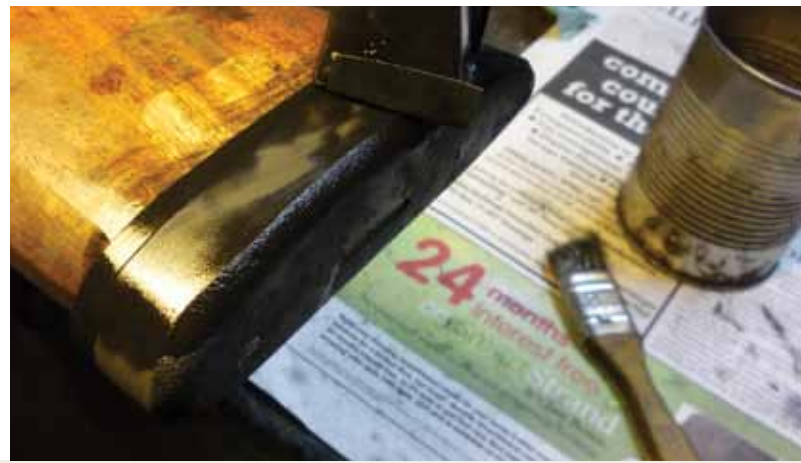
For hand-sanding to finish I use kerosene and 400-grit wet/dry paper to perform this task, with the pad set-up on an old dummy-stock.
