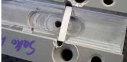
Measuring max reward travel against a known load. This works initially as a good visual comparison test, but findings can be used to calculate the recoil energy values for before and after comparisons.
