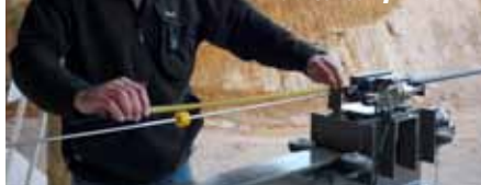
Testfiring 7mm Rem. Mag barrelled action on purpose-built testing machine.
